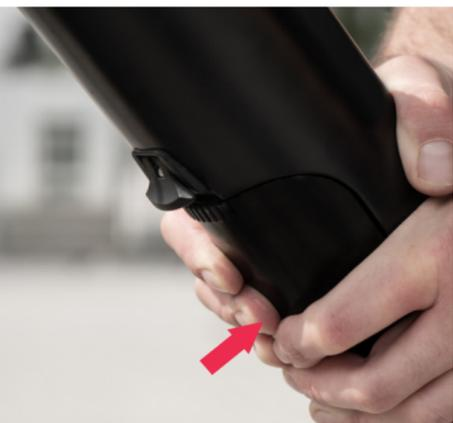
**1.** Press the Drivepack into the frame to unload the release mechanism
