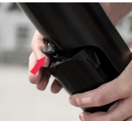
**3.** Gently tilt the lever back while simultaneously sliding the Drivepack into your second hand
