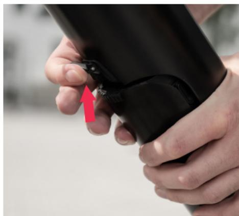
**2.** Pull the lever up to open the release mechanism
