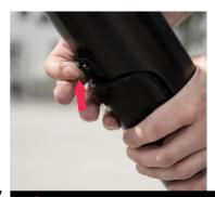
Pull the lever up to open the release mechanism
