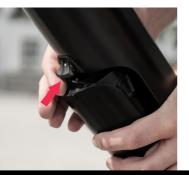
Gently tilt the lever back while simultaneously sliding the Drivepack into your second hand
