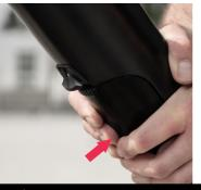
• Press the Drivepack into the frame to unload the release mechanism
